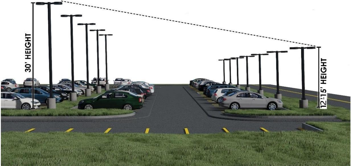
F. **Lighting Intensity Standards.** Figure 8.9.3: Specific Lighting Standards, defines specific standards for lighting intensity based upon the land use involved. Values are presented in allowable foot-candles (fc) maintained (measured horizontally) at grade and are to be averaged throughout the site to avoid hot spots and ensure minimum values at the edge of the development area.
